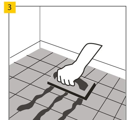
In the case of installation on the substrate covered with ceramic tiles, fill the tile joints with the gap wider than 4 mm and deeper than 1 mm with a durable compound for the filling of points, e.g. resin grout. Installation is allowed on tiles with grouts not wider than 5 mm and 1 mm deep without using levelling compound, provided the Multiprotec Hardlay or Vinclis Solid are used as underlay.
