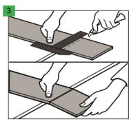
For additional cutting of floor panels, use a sharp knife, cut the top layer, then break the panel dynamically by leaning it on the edge. The floor panels may also be easily cut using an electric saw.
