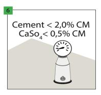
In the case of the cement grout, the moisture content in the substrate must be lower than 2.0%, and in the case of the anhydrite grout, it must be lower than 0.5%. In the case of installation with the underfloor heating, the abovementioned values must be 1.8% and 0.3% respectively.
