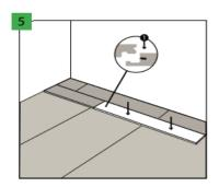
Then lower the panel in such a way as to fasten the lock on the short side, gently pressing the panel with fingers, starting from the corner and then towards yourself. The lock on the short side is provided with a special catch, which gets snapped if properly assembled. NOTICE! Do not use excessive force! If there are any difficulties with the lowering of the panel and closure of the lock, increase the clearance in the lock and lower the panel again.
