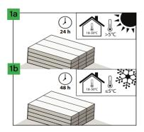
If the temperature is >5 °C during transport, the acclimatization time in a room with a temperature of 18-30 °C should be min. 24 hours. However, in case of temperature  $\leq\!5$  °C during transport, acclimatization time in a room with a temperature of 18-30  $^{\circ}\text{C}$  should be min. 48 hours.
