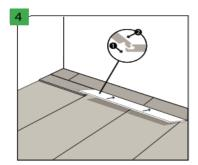
The Arbiton floor panels are provided with locks on the short and long side. First, connect the panel on the long side; for this purpose slide the long side of the panel into the groove of the previously installed row of panels. Move to the corner, leaving some clearance.
