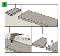
In the case of vertical pipes embedded in the substrate, leave free space around the pipes. Holes for the pipes must be drilled with a drill bit with a diameter that is bigger than the pipe diameter by 5 mm.
