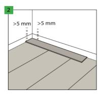
Leave 5 mm of perimeter space at the walls to allow the floor expansion. The maximum surface which can be laid without additional expansion joints is 200 m2. Above this surface, apply an additional expansion joint and enlarge all the expansion joints up to 10 mm. The maximum length of the floor surface in one direction, which can be laid without additional expansion joints is 20 m. Above this length, apply an additional expansion joint and enlarge all the expansion joints up to 10 mm.
