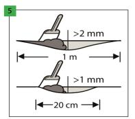
Make sure that the substrate is completely flat. All substrate irregularities exceeding 1 mm, with a length greater than 20 cm, or exceeding 2 mm with a length greater than 1 m must be levelled. Check if the use of the priming or sealing material is necessary. In order to prepare the substrate perfectly, spread the grout or the self-levelling compound on the entire surface.
