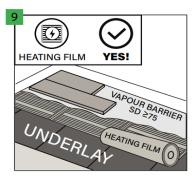
Installation on a heating foil is also allowed, provided that an appropriate underlay for the heating film and a vapor barrier foil SD ≥75 are used.
