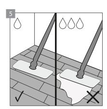
24 hours after the installation, it is possible to perform the "wet" cleaning of the floor, however, it is not allowed to install the installation mat in premises, which will be cleaned mechanically by means of a steam and/or water cleaner.
