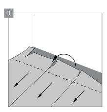
Peel back the protective layer which protects the adhesive. Do not remove the entire protective layer, but rather only a certain part of it that is necessary to position several LVT panels. After removing the protective layer, avoid contaminating the adhesive layer, as this will result in reducing the performance of the adhesive. Avoid walking or kneeling on the exposed layer of adhesive! The LVT panels must tight positioned on the installation mat tight to each other, without leaving any space.
