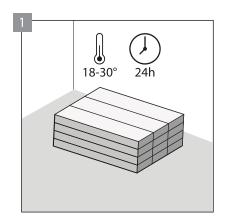
The installation mat should be stored at a temperature ranging between 5°C and maximum 35°C. Before the installation it should be subjected to the 48-hour acclimatisation at the temperature of 18–30°C, in the premises where it will be installed.
