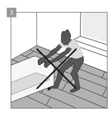
Directly after the installation, the floor may be walked upon gently, and heavy objects may be placed on the installed floor after 2 hours from the installation. The maximum adhesive strength is obtained after 24 hours following the installation; until that time, it is not recommended to move around any heavy objects or clean the floor.
