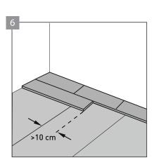
Start laying the floor from the smallest piece of underlay, ensuring a minimum 10 cm overlap on the adjacent installation mat. The laying of the first line of panels perfectly straight will affect the good visual effect of the whole room. The installer has up to 30 minutes to reposition any planks that have not been installed properly.
