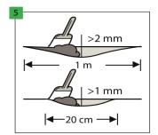
Make sure that the substrate is completely flat. All substrate irregularities exceeding 1 mm, with a length greater than 20 cm, or exceeding 2 mm with a length greater than  ${\bf 1}\,{\rm m}$  must be levelled. Check if the use of the priming or sealing material is necessary. In order to prepare the substrate perfectly, spread the grout or the self-levelling compound on the entire surface.
