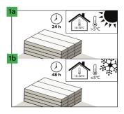
If the temperature is >5  $^{\circ}\text{C}$  during transport, the acclimatization time in a room with a temperature of 18-30  $^{\circ}\text{C}$  should be min. 24 hours. However, in case of temperature  $\leq$ 5 °C during transport, acclimatization time in a room with a temperature of 18-30 °C should be min. 48 hours.
