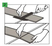
For additional cutting of floor panels, use a sharp knife, cut the top layer, then break the panel  $% \left\{ 1,2,\ldots ,2,\ldots ,2,\ldots \right\}$ dynamically by leaning it on the edge. The floor panels may also be easily cut using an electric saw.
