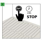
Before installation, turn off the underfloor heating for 24 hours.
