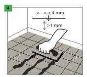
In the case of installation on the substrate covered with ceramic tiles, fill the tile joints with the gap wider than 4 mm and deeper than 1 mm with a durable compound for the filling of points, e.g. resin grout.
